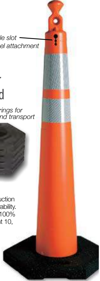
Grabber-Cone 42" with (1) 4" and (1) 6" band of white reflective sheeting and a 16 lb. recycled rubber base
