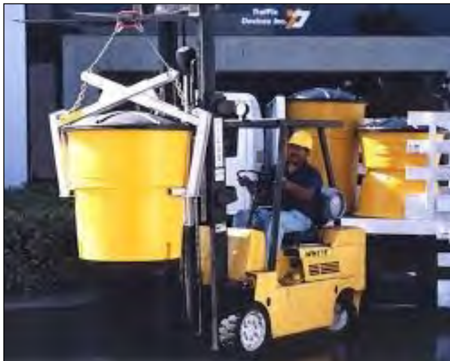
Figure 11: Forklift with attached Lifting Ring moves 1400 lbs. filled sand barrel
