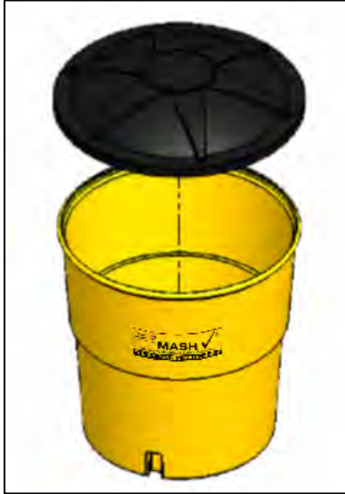
Figure 8a: 1400 lbs. Barrel Assembly.
