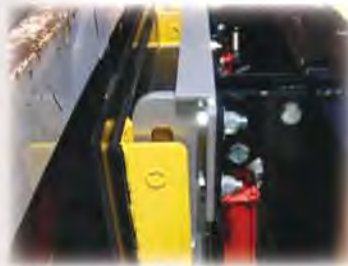
Align hooks over bars
