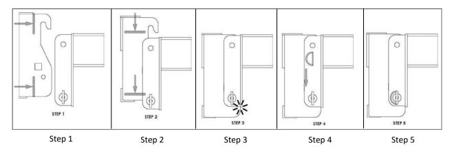
Be sure that the Hook on the TMA side is above the Pin on the Truck Side. Adjust accordingly if necessary. With the securing Pins and Clips removed from the Truck side, push the TMA up to the Truck Mount.
