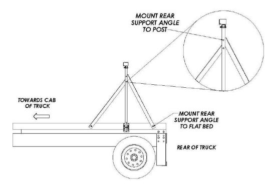
6. When the TMA is raised to the stored position, the wear plates that are mounted onto the top half of the Cartridge tubes (already mounted onto TMA) should align and rest upon the top support post saddles (P/N 11040C) as shown in the figure below.
