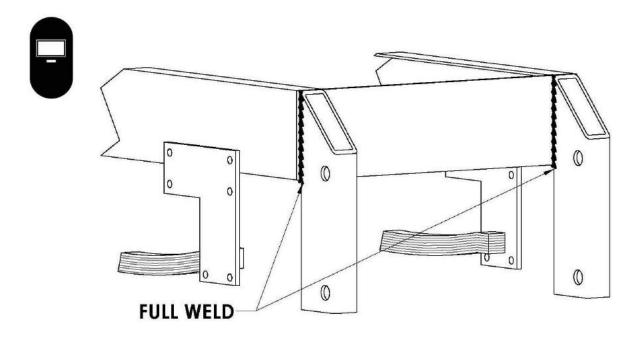
6. Position the splice plates, as shown here in this figure below, against the sides of the frame and the vertical tubes. Mark on the plate the position of two holes for ¾" bolts. Drill these holes in the plates and the frame. Weld the edge of the plate to the vertical tube. The truck frame weld areas should be spray painted to prevent rust.
