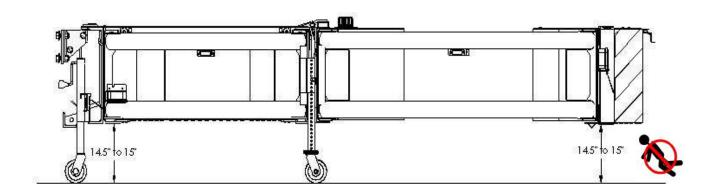
4. With the jacks deployed, roll the deployed TMA to the rear of the host vehicle and align the TMA centerline with the vehicle, as shown in the following figure. The backing plate that is bolted onto the TMA (See step 2) should be flush with the ends of the truck frame.
