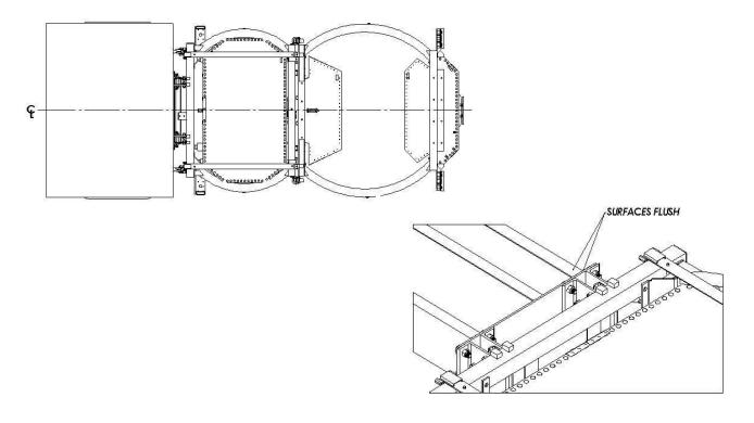
5. After proper confirmation of the backing plate being level and 90° to the horizontal surface, deploy the drops jacks and unbolt the TMA from the backing plate that is already tacked onto the host vehicle. Fully weld the backing plate on both the inside and outside of the frame rails. Proper welding locations are specified in the figure below:
