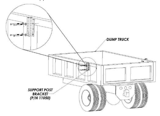
2. Insert the support post (P/N 11055NJ) into the support bracket. Adjust the post to the appropriate height, which will vary based on the height of the dump truck of the host vehicle, to where the cartridge tubes will be able to rest on the support post top saddle when the TMA is in the stored position. This figure below illustrates how the support posts can be adjusted upon installation.
