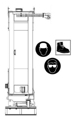
5. Use the forklift to lower the pallet to the horizontal position as shown in the figures below. Verify that the pallet is tipped in the correct orientation with the junction box on top, which can also be seen in the following figure. Caution – Keep personnel away from the TMA when the steel bands are cut. Keep clear from pallet when pallet is pulled free of the cartridge for it will drop a few inches. Steel band locations are identified in the figures below.
