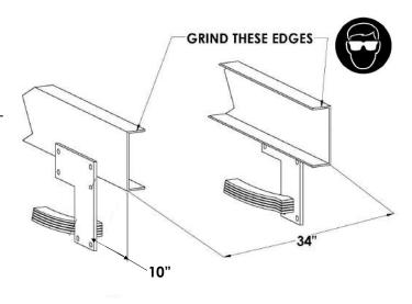
2. A backing plate (33" x 10") should be centered on the back of the truck frame. Note where the frame will be welded to the plate and grind the plate in this location. Tack weld the rear plate into position and make sure that the rear plate is positioned vertically at 90° to horizontal. Continue by welding the inside of the frame end to the plate.
