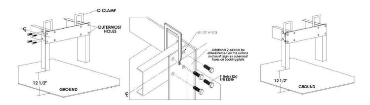
7. Weld the angles in place at the rear of the angle. Refer to the figure below for proper welding locations.
