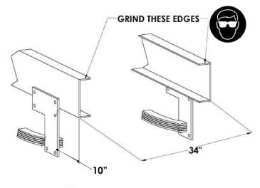
2. Mount the Backing Plate (P/N: 10353) onto the backup of the TMA as shown in this figure (right). Mounting the backing plate onto the TMA will simplify the alignment process when mounting the backing plate onto the truck frame of the host vehicle.
