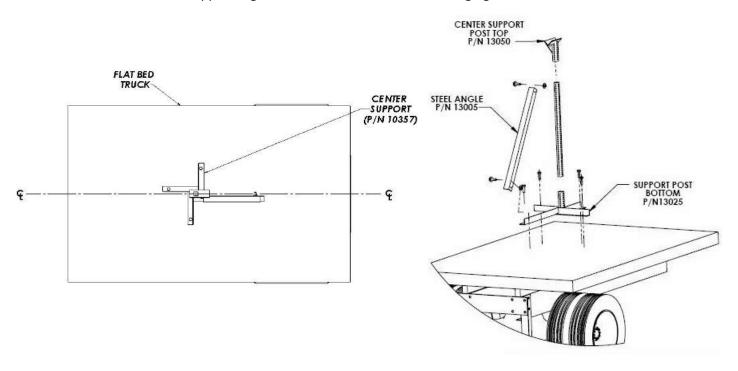
2. Make sure the angle located on the rear cartridge diaphragm aligns with the center support top post angle when the TMA is in the stored position, as shown in this bottom figure.
