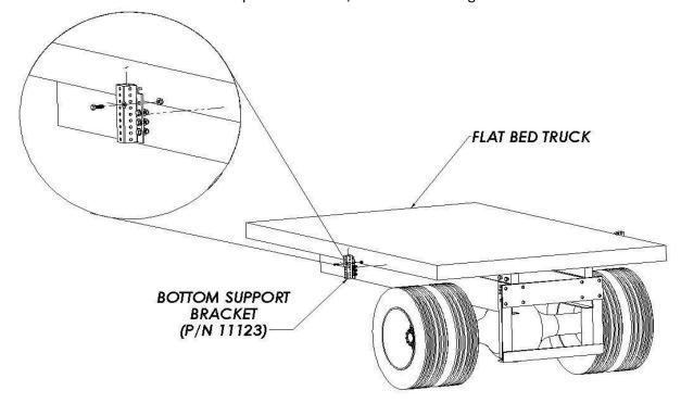
2. Insert the support post into the bottom support bracket. Adjust the post to the appropriate height, which will vary based on the host vehicle, to where the Cartridge tubes will be able to rest on the support post top saddle when the TMA is in the stored position. This figure below illustrates how the support posts can be adjusted upon installation.
