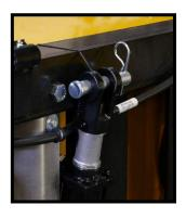
8. Remove the clevis and hair pins from the hydraulic cylinder.
