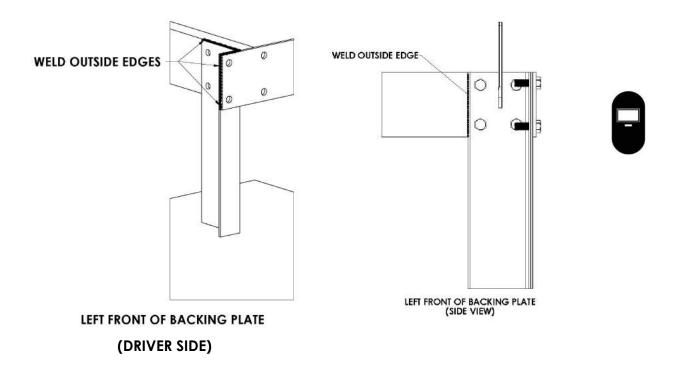
8. Install the lower bottom angle (P/N: 10356) and fully weld the angle in place. Refer to the following figure for proper welding locations.
