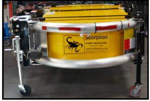
8. Cut and remove the zip ties that hold the hydraulic cylinders to the Strut. Remove the hair pins and clevis pins from both cylinders. \*Clevis pins and hair pins are needed later on in assembly. Once the hydraulic cylinders are free of the strut, grab the end of the cylinder and lift until the cylinder is fully extended.
