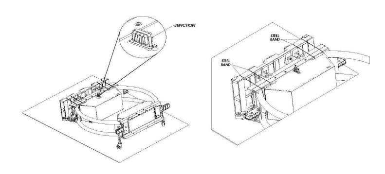
6. Use the forklift to lift the backup end of the cartridge to a sufficient height to deploy the swivel jacks located on the backup as shown in following figure. Crank the swivel jacks and rotate the wheels to the deployed position.
