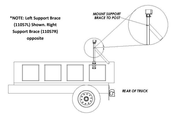
4. Pivot the support brace towards the rear end of the truck. Mark and drill another hole into the dump truck and securely fasten the brace in place, as shown in the figure below.
