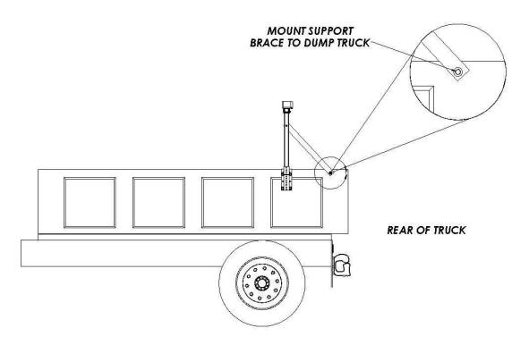
5. When the TMA is raised to the stored position, the wear plates that are mounted onto the top half of the cartridge tubes (already mounted onto TMA) should align and rest upon the top support post saddles (P/N 11040C) as shown in this figure below.
