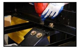
Lock out Arm Bolted **Onto Cartridge**
