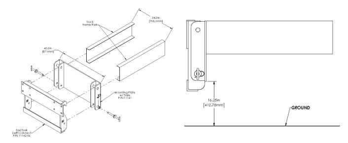
Figure 1: Exploded and assembled view of Configuration 1.
