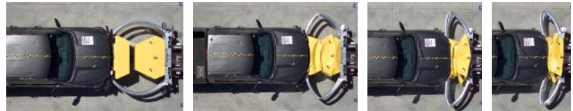
Scorpion II ® Metro TL-2 TMA Impacted by 5,000 lbs (2,268 kg) Pick-Up Truck
