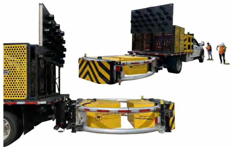
Scorpion II ® Metro TL-2 TMA Impacted by 5,000 lbs (2,268 kg) Pick-Up Truck
