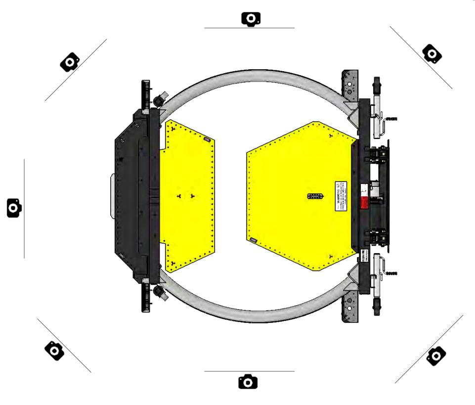
Please provide photos of the Metro TMA taken at the approximate angles shown. The views depicted are required at a minimum for Traffix Devices to assess the damage and make repair recommendations. If any gouges, indentations, or cracks on the tube assemblies are discovered during the inspection, closeup photos should be taken.
