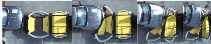
Scorpion II® TL-3 TMA Impacted by 5,046 lbs (2,289 kg) Pick-Up Truck
