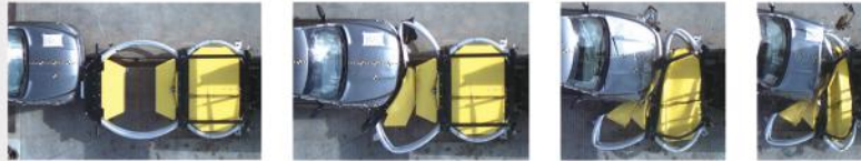
Scorpion II ® TL-3 TMA Impacted by 5,046 lbs (2,289 kg) Pick-Up Truck
