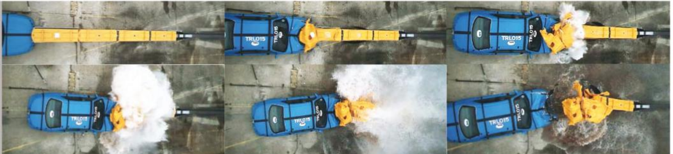
Tested and Passed: EN1317-4 P4 Impact Speed: 110 Km/h Vehicle Type: 1500 kg Bullet Vehicle Impact Angle: Head-On Centre
