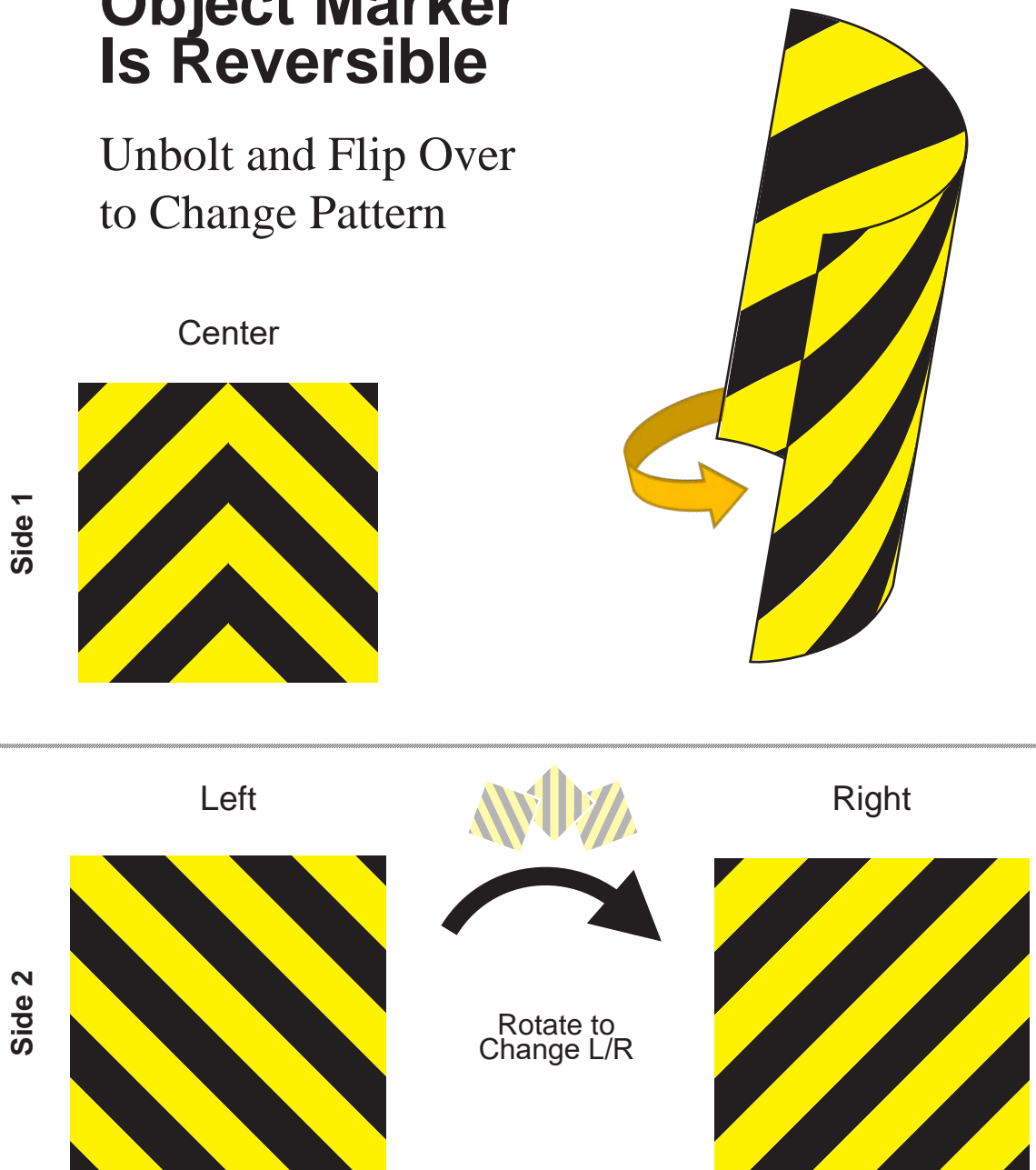
Figure 18: SLED Object Marker Installation
