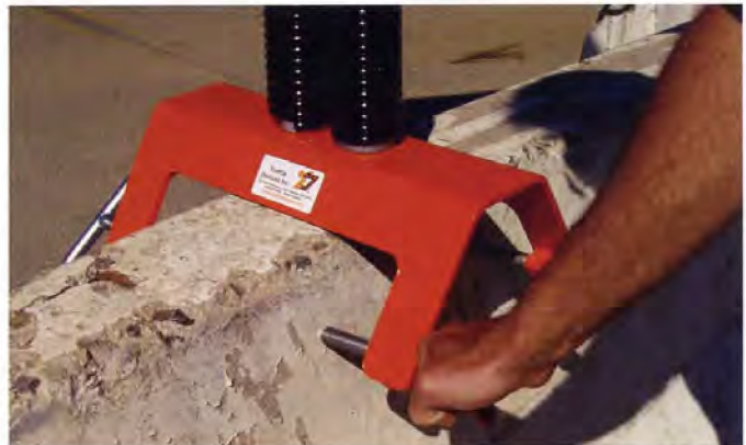
T-pins with hardened steel points secure stand to concrete barrier wall
