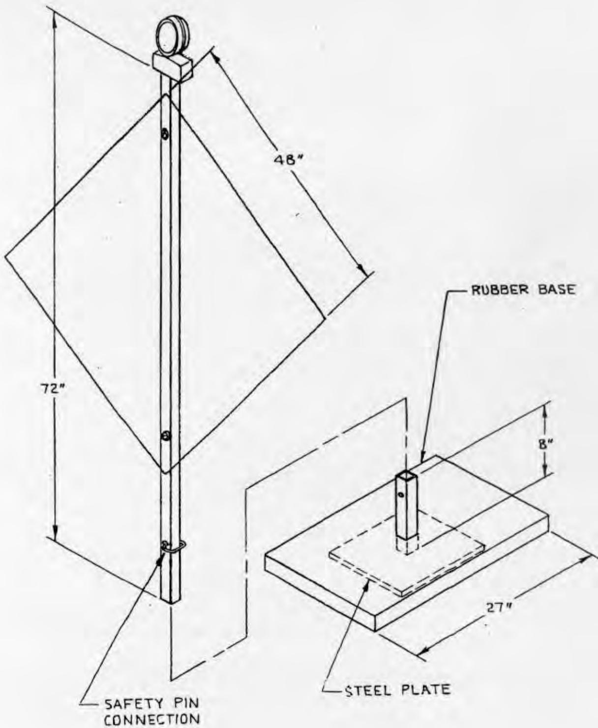
Figure 5. - Rubber Base Sign Stand with Pinned Inner Mast, Forty-eight Inch by Forty-eight Inch Aluminum Sign, and B-Light; Sign Height Twelve Inches Above Ground
