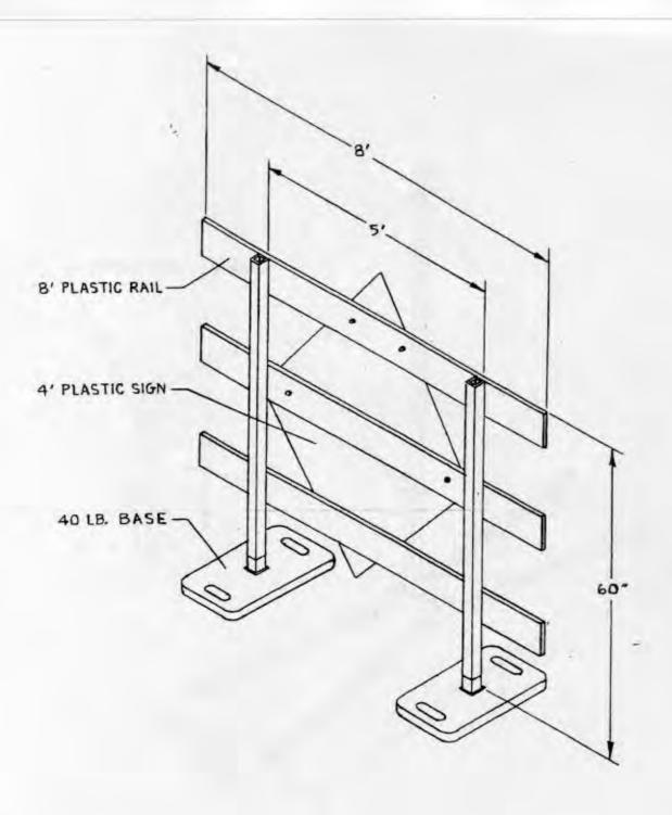
Figure 2. – Type 3 Plastic Barricade with Plastic Posts and Pinned Rubber Bases, Forty-eight Inch by Forty-eight Inch Corrugated Plastic Sign; Sign Height Twelve Inches Above Ground.
