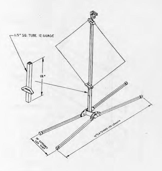
Figure 3. – Econo Buster Sign Stand with Forty-eight Inch by Forty-eight Inch Aluminum Sign with Slip-over Outer Tube Mast; Sign Height Sixteen Inches Above Ground.
