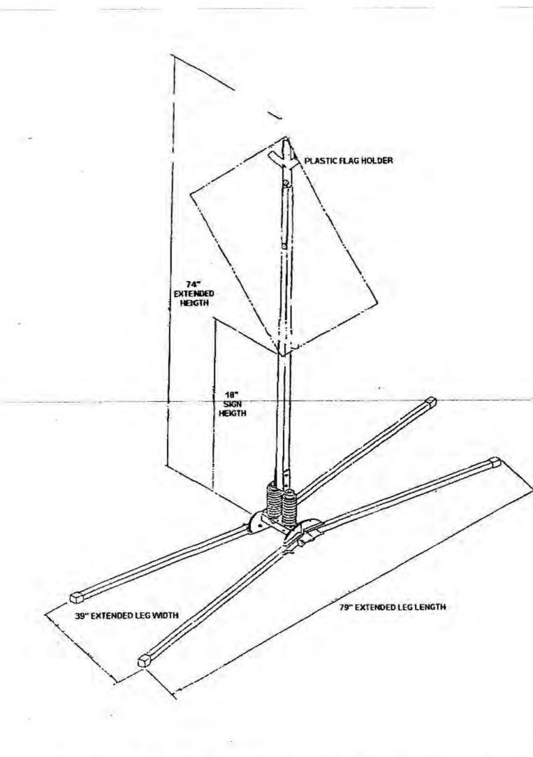
Figure 3. – Aluminum Buster Sign Stand with Forty-eight Inch by Forty-eight Inch Aluminum Sign Bolted to Inner Mast and Plastic Flag Holder; Sign Height Eighteen Inches Above Ground.
