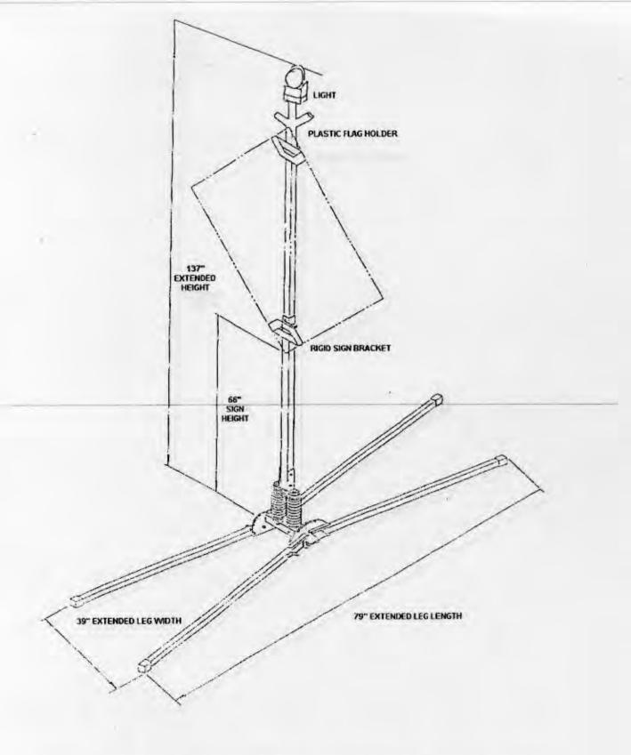
Figure 2. – Big Buster Sign Stand with Forty-eight Inch by Forty Eight Inch Aluminum Sign, Aluminum Inner Mast, and Plastic Flag Holder; Sign Height Sixty-six Inches Above Ground.
