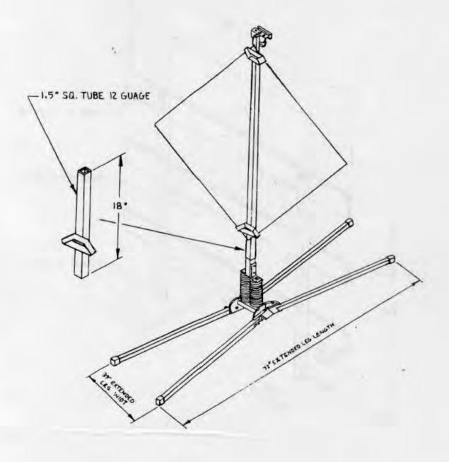
Figure 1. – Little Buster Sign Stand with Forty-eight Inch by Forty-eight Inch Aluminum Sign with Slip-over Tube Mast; Sign Height Eighteen Inches Above Ground.
