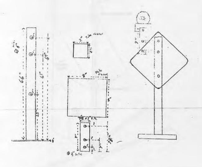
Figure 1. - Rubber Pole Base with 40 lb. Ballast, Thirty-six Inch by Thirty-six Inch Aluminum Sign, and Light.
