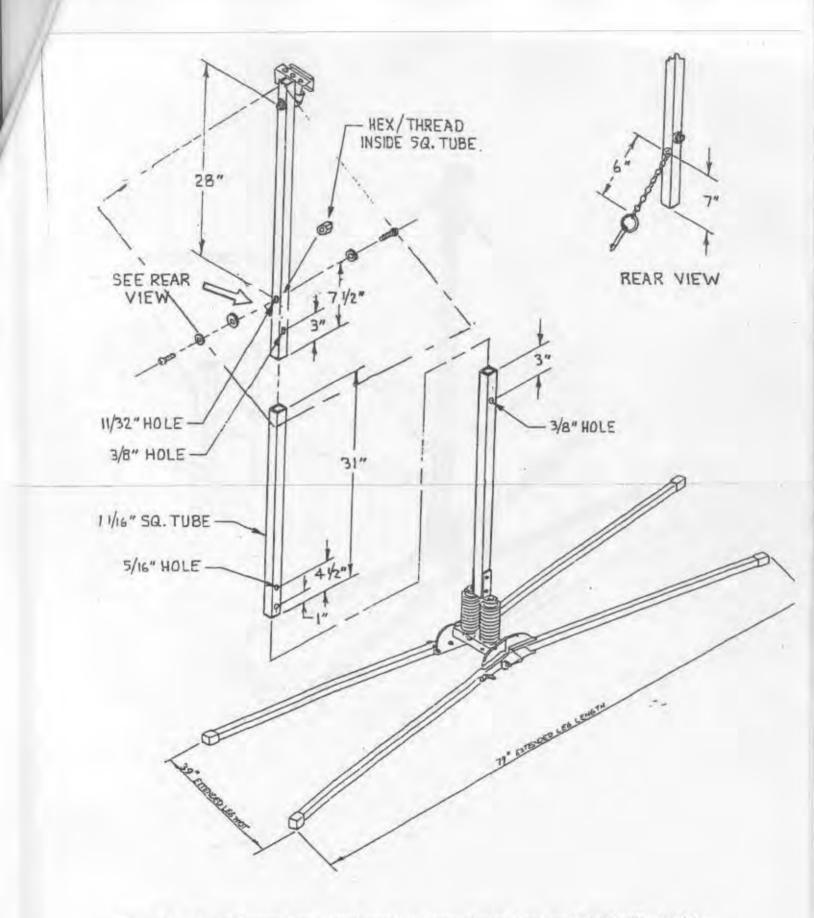
Figure 4. – Little Buster Sign Stand with Full Length Inner Mast and TrafFix Flag Holder; Sign Height Eighteen Inches Above Ground.
