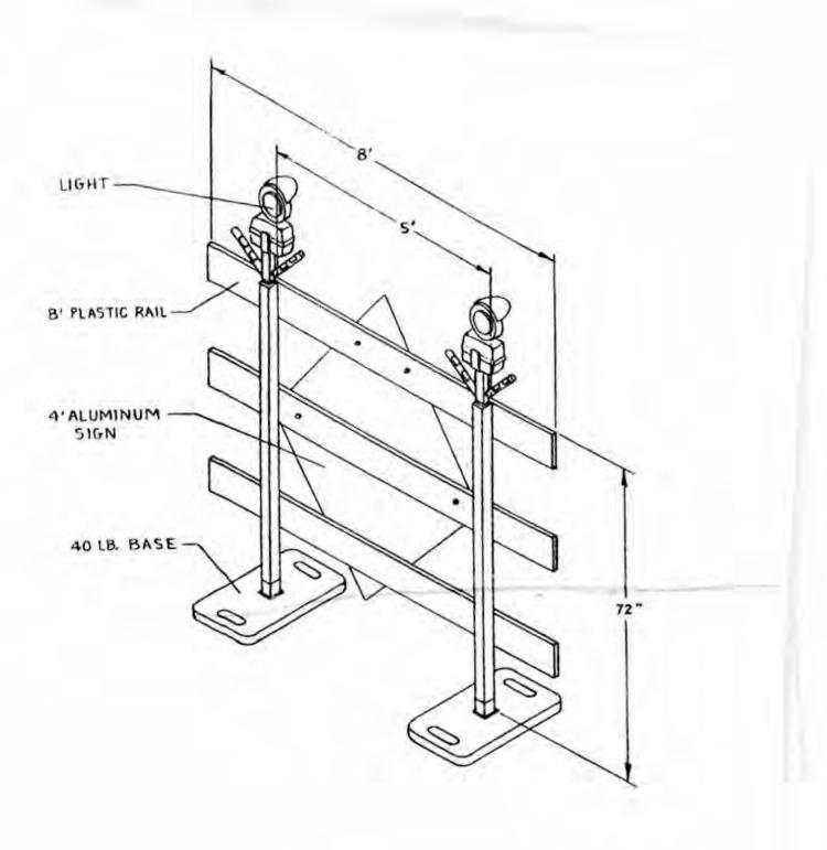
Figure 4. – Type 3 Plastic Barricade with Steel Post Uprights with Lights, Forty-eight Inch by Forty-eight Inch Aluminum Sign; Sign Height Twelve Inches Above Ground.
