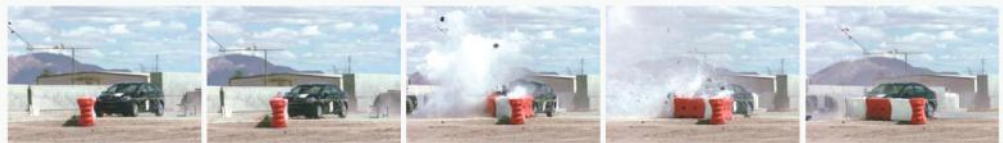
TraFFix Water-Cable Barrier® TL-2 Impacted by a 2,505 lb. (1,113 kg) KIA Rio at 44 MPH (70 KPH)
